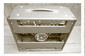
Controls are: Volume, Treble, Midrange, Bass, Master Volume, Cut and Reverb, and all are very effective in shaping the tone of the amp. Sustain and distortion are dialed in with the level of the Master Volume. The Z is an exceedingly expressive amp, with an exceptionally smooth overdriven tone. The four EL84s and the Celestion speaker create a lush and rich tone that is unmistakable – a classic tone that simply can't be beat for rock and blues.
